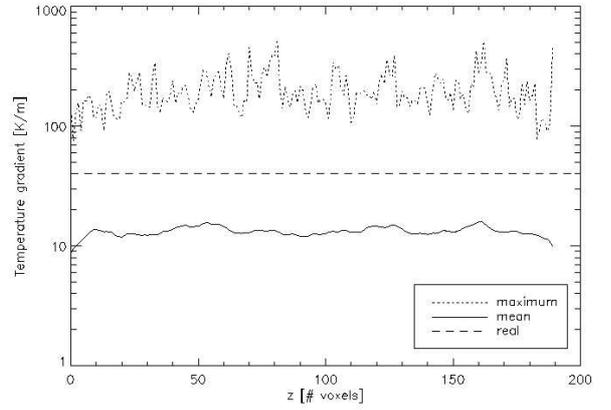
Figure 8. For each  $x, y$ -voxel plane, along the  $z$ -direction, maximum and mean computed temperature gradients for the ice matrix of the sample at day 0. The overall applied temperature gradient was  $40 \text{ K m}^{-1}$ .
