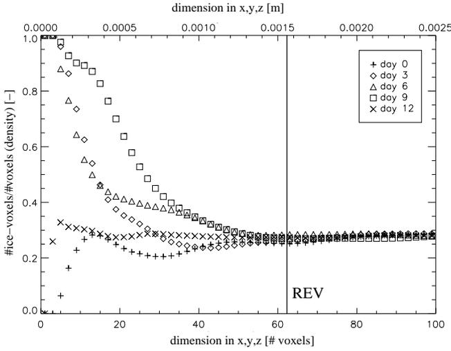
Figure 2. The fraction of ice-voxels, which is proportional to the density, in function of the size of cubic sub-volumes of the computational domain  $\Omega$ , for the microstructure every three days during the experiment.
