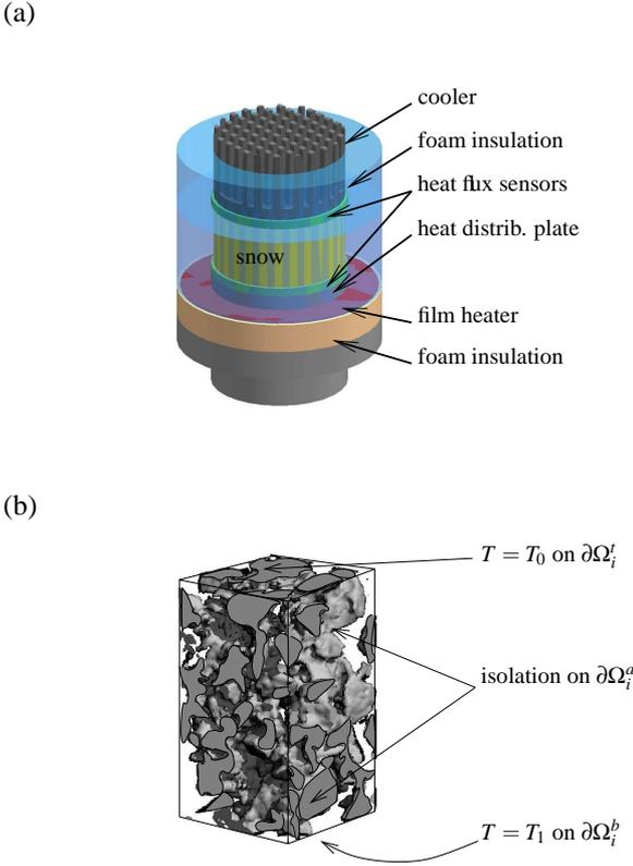
Figure 1. The temperature-controlled snow breeder (a). The snow-chamber had a diameter of 50 mm and a height of 23 mm. (b) The subdomain ( $2.5 \times 2.5 \times 4.75$  mm) used for the numerical computations.
